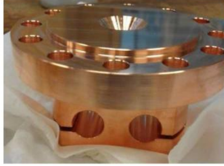
FIGURE 3.4: Photo of the cold finger flange, which sits in the bottom of the LN2 tank.
