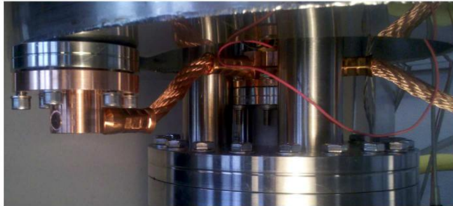
FIGURE 3.6: Photo of the cold lines (copper cable) connecting the cold finger in the inner cryostat (right) with the cold finger (left) on the LN2 tank (top).
