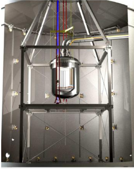
(A) Image illustrating the XENON1T experiment with its TPC and cryostat in the Cherenkov water muon veto.
